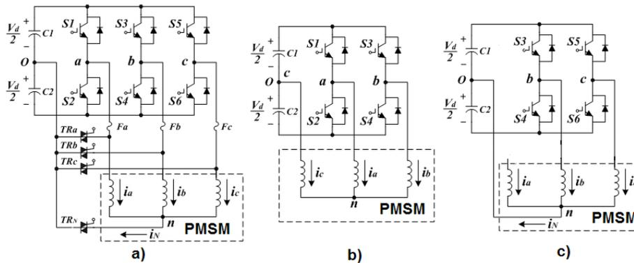
Fig. 1 Fault tolerant inverter: a) basic topology, b) failure of transistor leg, c) failure of motor phase
