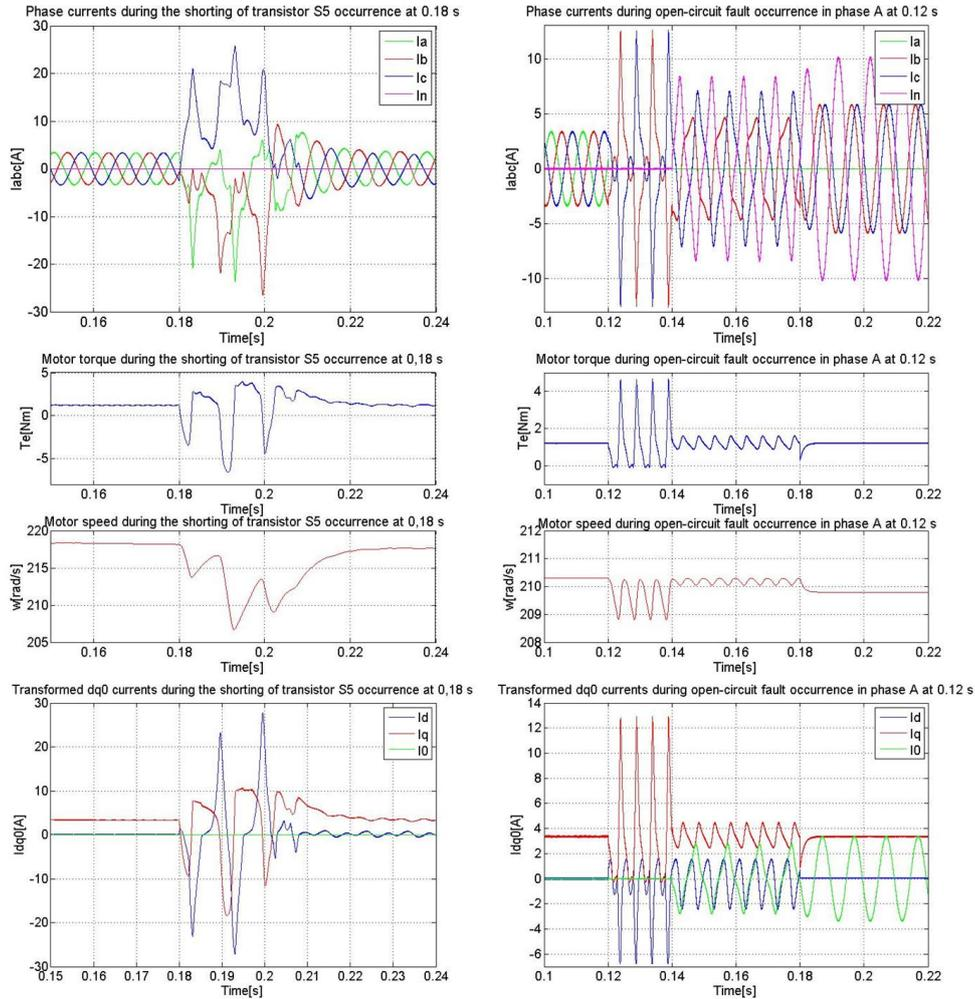
Fig. 4 Fault tolerant control for topology 4S3P (left side) and topology 4S2P (right side)
