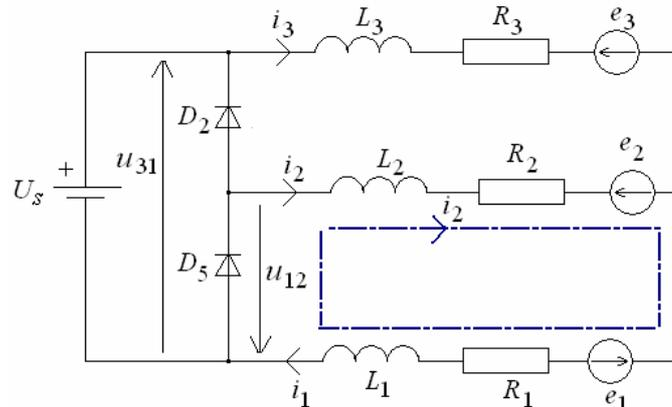
Fig. 5. The equivalent electric circuit for IV stage of converter
