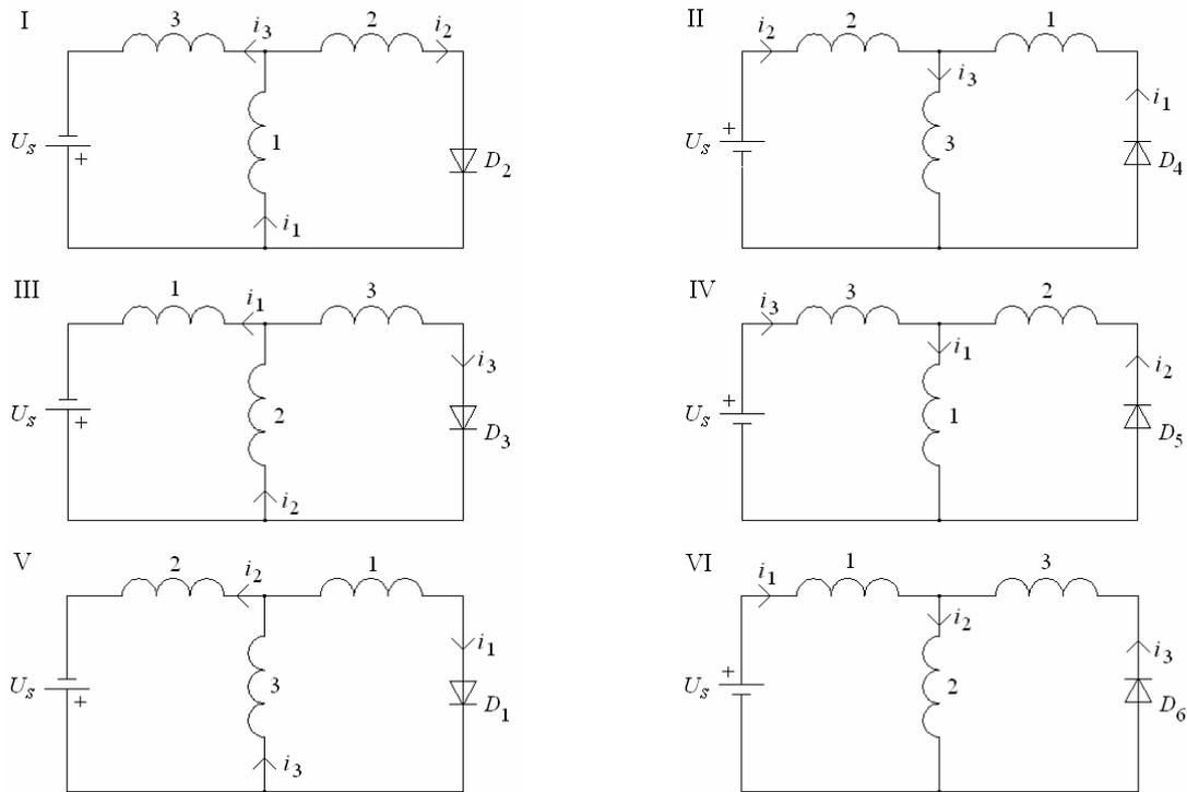
Fig. 4. The stator winding connection in the six converter states
