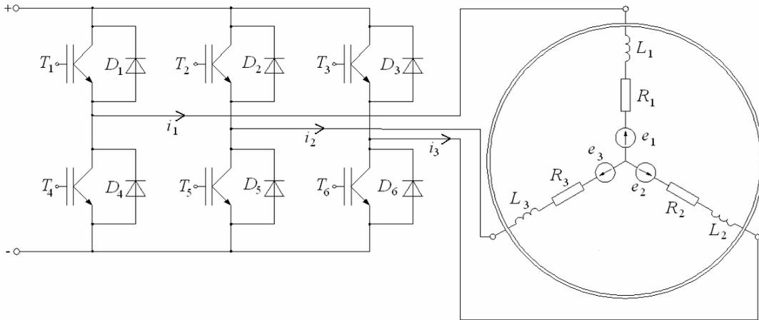
Fig. 2. The conventional six-switch converter connected with motor circuit model
