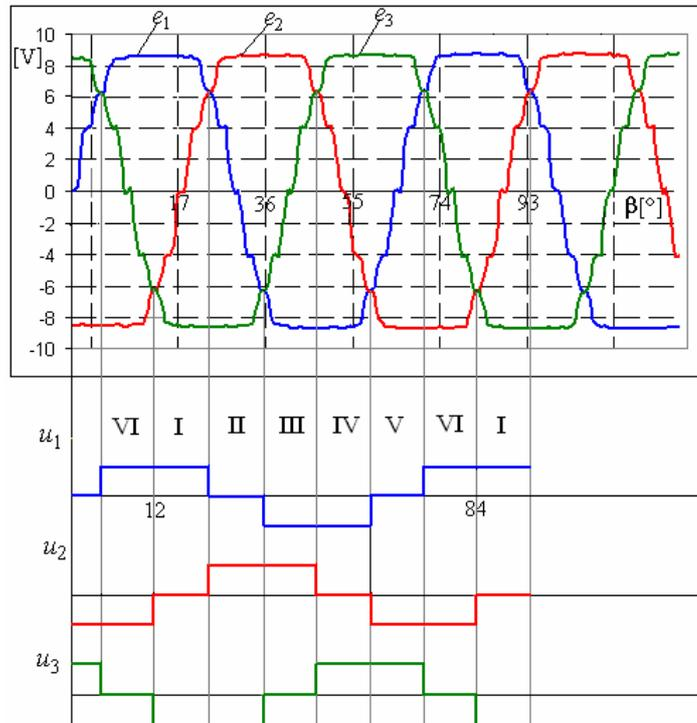
Fig. 3. Calculated back EMF and voltage waveforms of load machine
