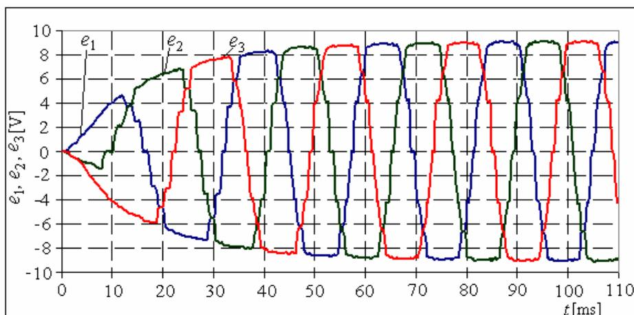
Fig. 6. Back EMF waveform
