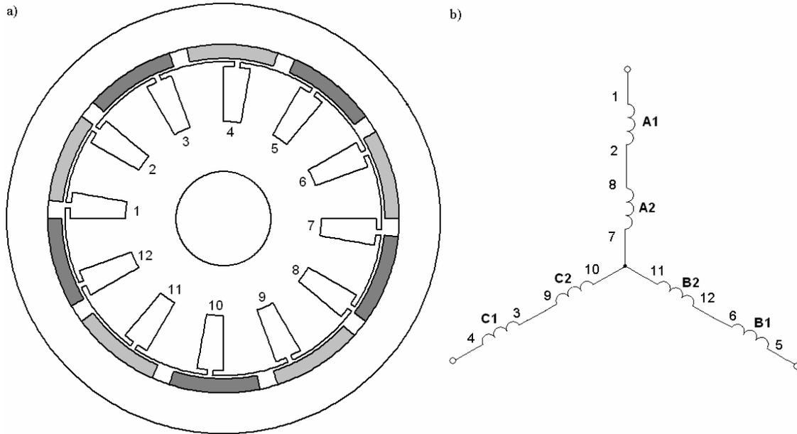
Fig. 1. The outer rotor permanent magnet brushless DC machine (a) and the stator winding configuration (b)
