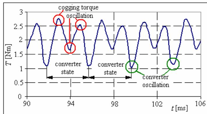
Fig. 10. Oscillations in torque waveform
