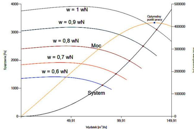
Fig. 3. Fan and system flow characteristics
