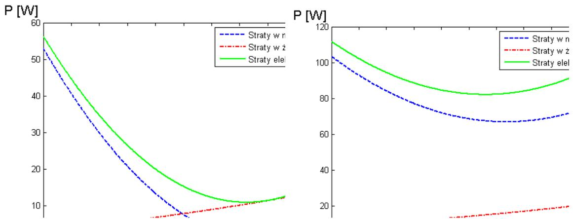
Fig. 7. Losses (copper, core and total) as function of  $i_{od}$  current. Speed equals  $\omega$  (left side) and nominal ( $1.7[Nm]$ , right side)
