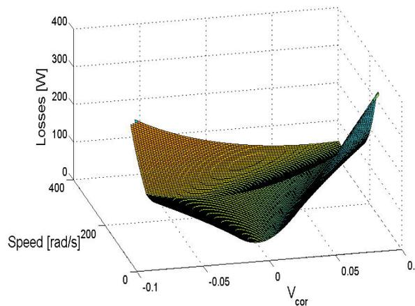
Fig 14. Power losses versus speed and correction voltage
