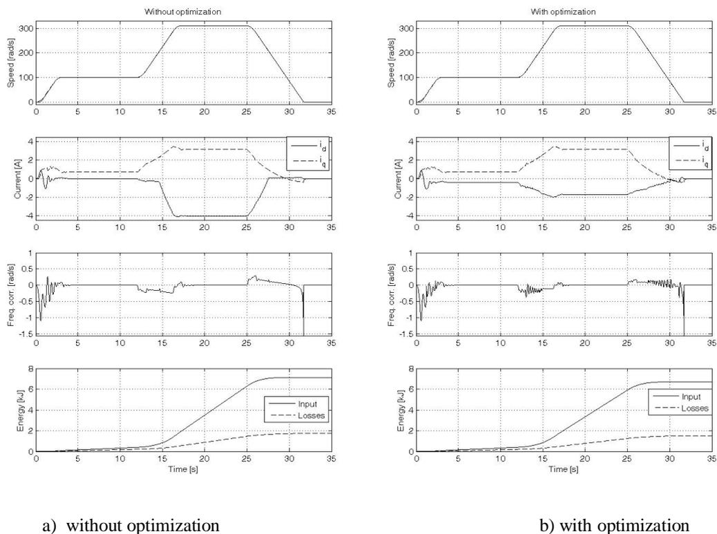
Fig. 15. Simulation results for system without/with optimization block.
