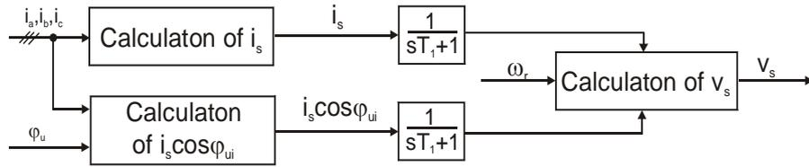
Fig 11. The algorithm for calculating the voltage  $v_s$
