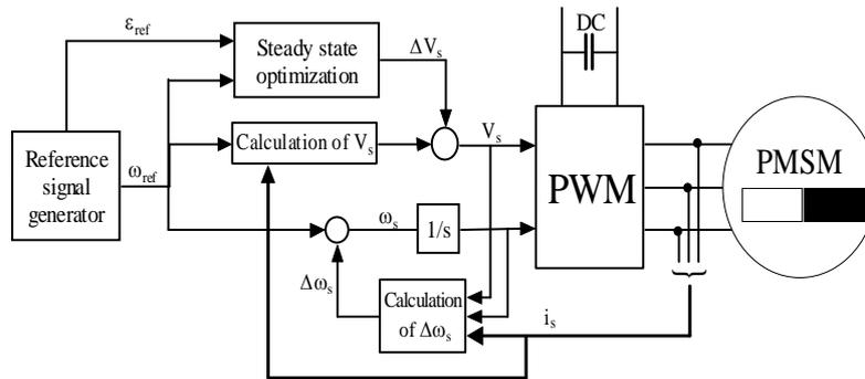
Fig 13. Structure of PMSM drive with stabilizing loop and steady state optimization
