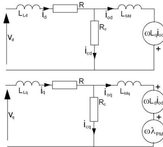
Fig. 1. Direct and quadratic axis equivalent circuits of PMSM
