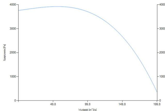
Fig. 5. Fan flow characteristic
